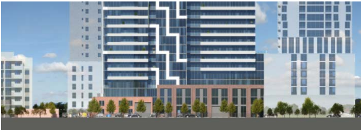
Figure 69: North Elevation enlarged detail of the proposed development showing the reconstructed façade of Radigan Building, G+C Architects, June 2023.
