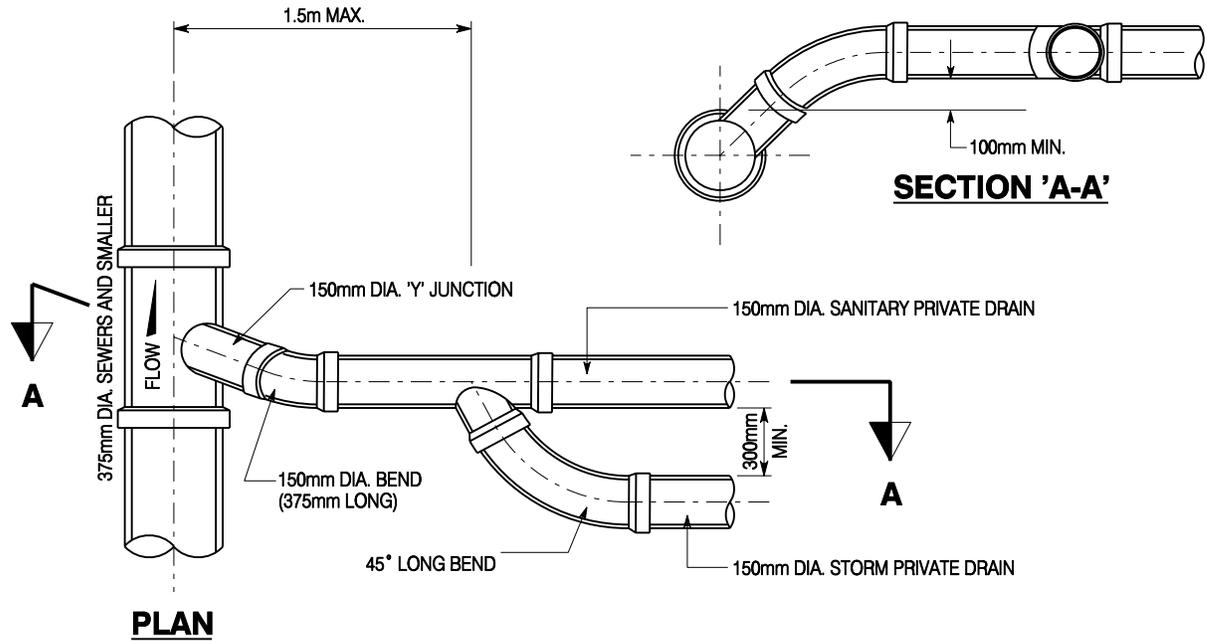
**CONNECTION TO 375mm DIA. SEWERS AND SMALLER**
